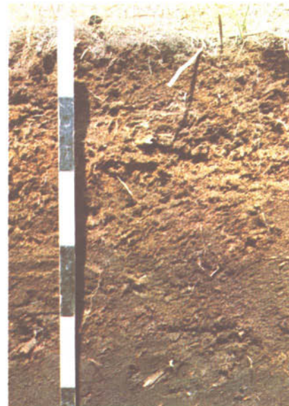
Soil profile of Stead Series. A Typic Mesisol developed on deep, moderately well decomposed herbaceous fen peat. Note thin sphagnum cap on the surface.
