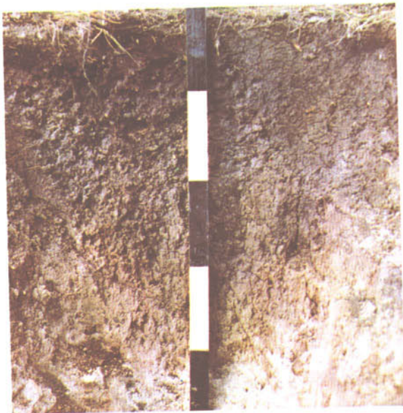
Soil profile of Homebrook clay. An Orthic Dark Grey soil developed on moderately to strongly calcareous fine textured till.
