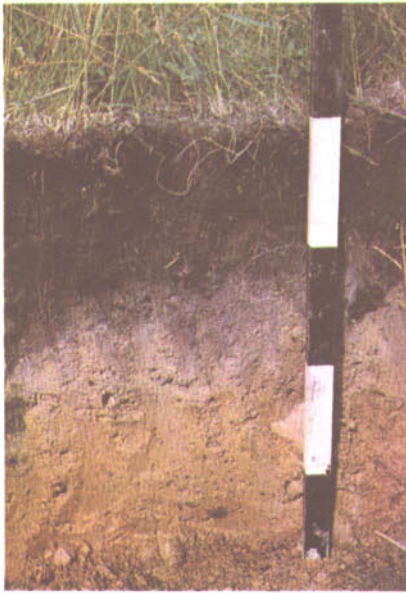
Soil profile of Lundar loam. A thin Gleyed Carbonated Rego Black soil developed on extremely calcareous glacial till.
