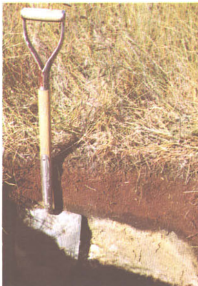
Soil profile of Meleb loam, peaty phase. A Carbonated Rego Humic Gleysol developed on extremely calcareous glacial till.
