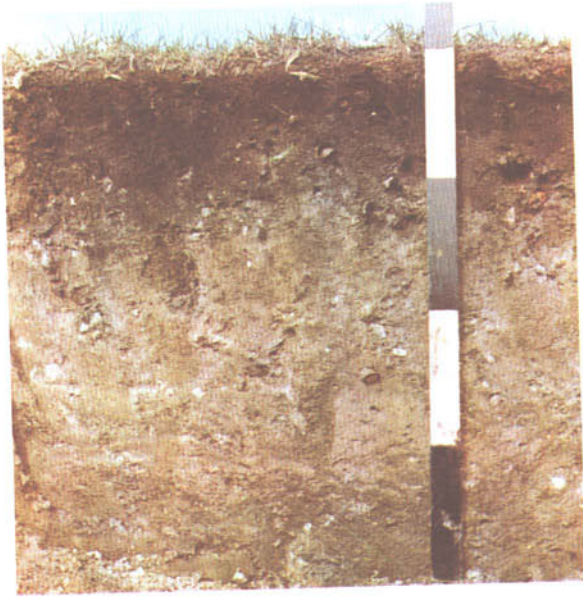
Soil profile of Inwood loam. A thin Gleyed Dark Grey soil developed on extremely calcareous glacial till.
