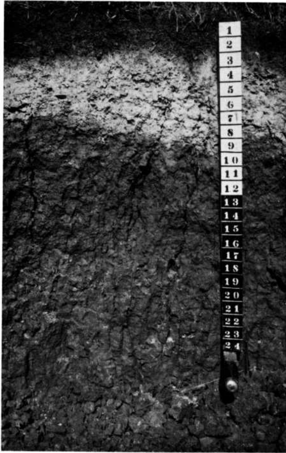
A profile of the Smithville silt loam The Ae horizon is developed within the surface silt loam and lies directly on the massive clay. The dark brown Bt horizon extends to a depth of 18 inches.
