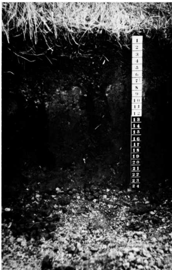
A profile of the Lincoln clay These clay soils are massive, and when dry possess vertical cracks with large prismatic structures.
